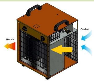
The device works on the principle offorced convection. The air flow is forced fan. Cold air is drawn in the back of the unit. Further washes flowing from the heater receives heat. The heated air is expelled in front of the heater. The device has a thermostat for the regulation temperatury 5-35 oC. The unit area equipped with thermal protection is acting automatically. The unit features: ventilation, heating with half the power, heating at full power. Device has cooling thermostat.
